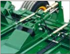
Maintenance free suspension removes shock loading and stress
