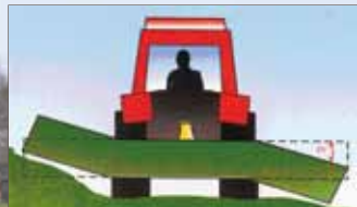
The wings float up to 25° above and below the cutting plane
